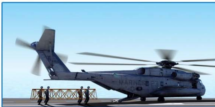
Entire truss and ducted rotors fit in cargo hold of a CH-53E
